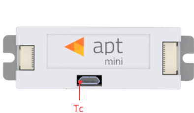
T_c is measured on metal sleeve of micro-USB programming port in location specified above
