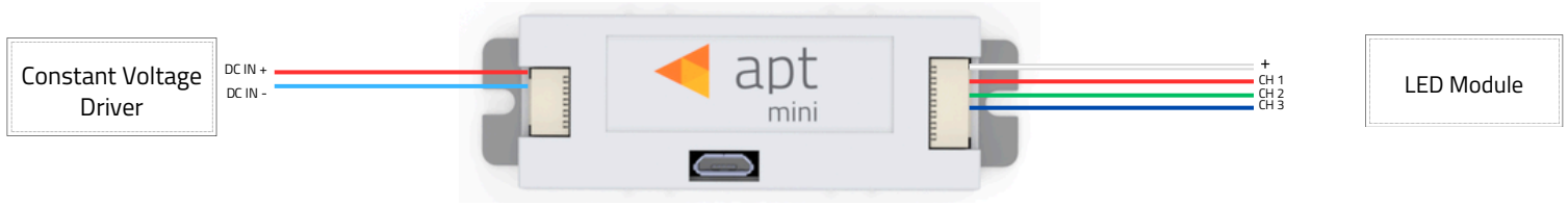
Figure 9 – APT3-VWC-M2 Wiring Diagram
