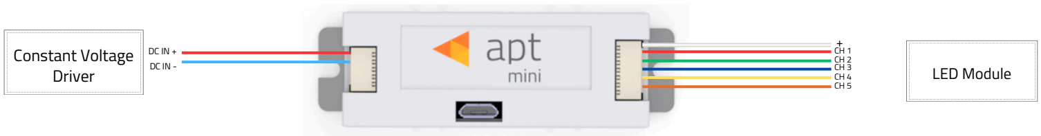
Figure 10 – APT5-VWC-M2 Wiring Diagram
