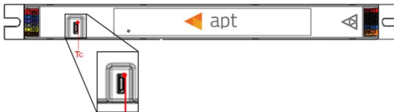
Fig. 4 - Tc is measured on metal sleeve of micro-USB programming port in location specified above
