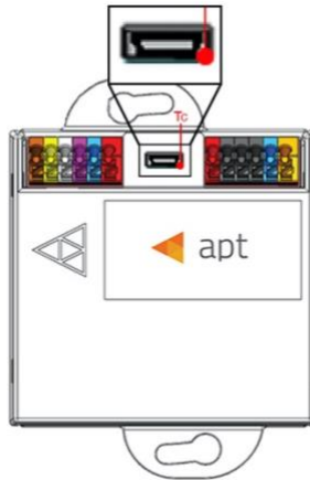
Fig. 4 - Tc is measured on metal sleeve of micro-USB programming port in location specified above
