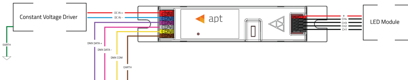
Figure 2 - APT-CV4-VA-LN-CVO DMX512/RDM Configuration
