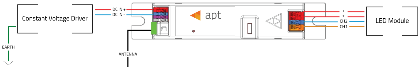
Figure 5 - APT-CV2-VWx-LN-CVO Wireless Communication Configuration
