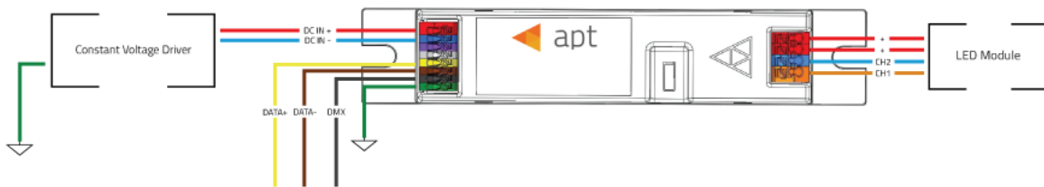
Figure 2 - APT-CV2-VA-LN-CVO DMX512/RDM Configuration
