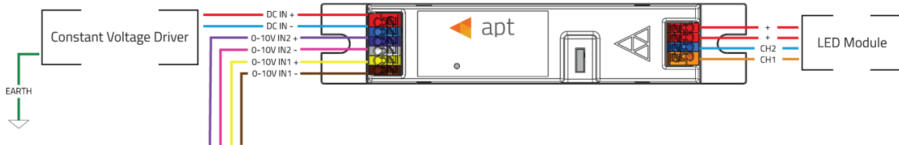
Figure 4 - APT-CV2-VC-LN-CVO Dual 0-10V Dimmer Configuration
