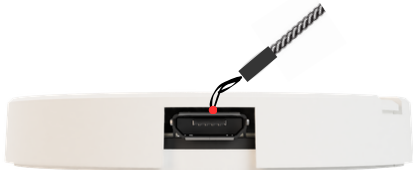
Figure 2 - USB Tc temperature is measured on the metal sleeve of the micro-USB programming port. To measure USB Tc, insert a K-type thermal probe between micro-USB and top encasement of the ORB controller as shown. Solder the tip of the thermal probe to the center of the USB connector.
