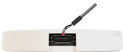
Figure 2 - USB Tc temperature is measured on the metal sleeve of the micro-USB programming port. To measure USB Tc, insert a K-type thermal probe between micro-USB and top encasement of the ORB controller as shown. Solder the tip of the thermal probe to the center of the USB connector.
