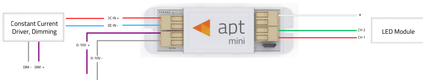
Figure 5 – APT-CC3-VS-M1-xxxxTW2 Wiring Diagram
