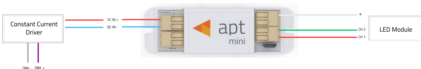
Figure 7 – APT-CC3-VS-M1-xxxxSW2 Wiring Diagram
