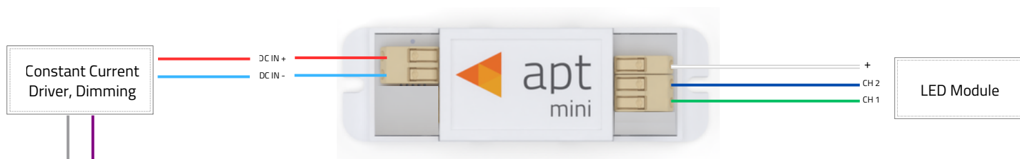
Figure 2 – APT-CC-VDW-M1-xxxx Wiring Diagram
