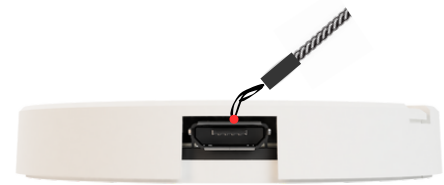
Figure 1 - USB Tc temperature is measured on the metal sleeve of the micro-USB programming port. To measure USB Tc, insert a K-type thermal probe between micro-USB and top encasement of the ORB controller as shown. Solder the tip of the thermal probe to the center of the USB connector.
