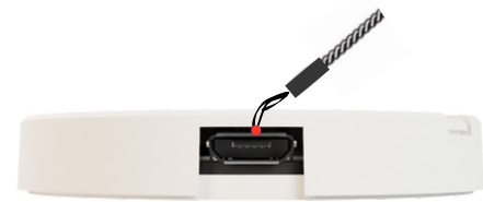
Figure 1 – USB T c temperature is measured on the metal sleeve of the micro-USB programming port. To measure USB T c , insert a K-type thermal probe between micro-USB and top encasement of the ORB controller as shown. Solder the tip of the thermal probe to the center of the USB connector.
