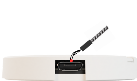
Figure 1 – USB Tc temperature is measured on the metal sleeve of the micro-USB programming port. To measure USB Tc, insert a K-type thermal probe between micro-USB and top encasement of the ORB controller as shown. Solder the tip of the thermal probe to the center of the USB connector.
